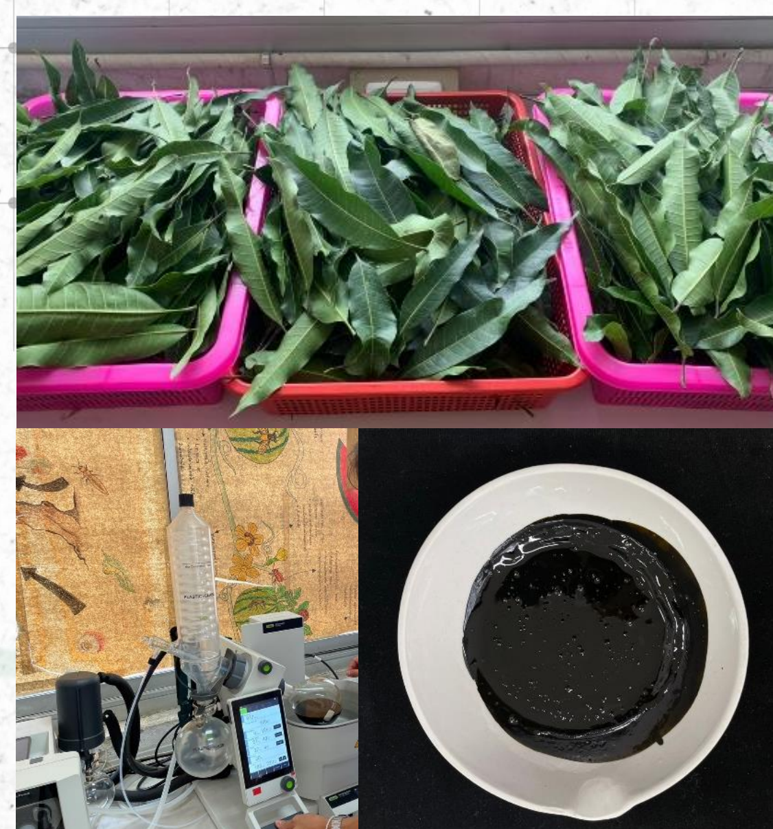
Figure 3 Extraction of allelopathic substances from mango leaves
